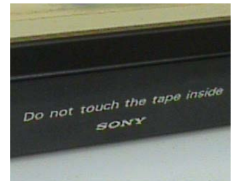
(White lettering on door- Note: Sony with blue lettering does not usually have sticky shed)
